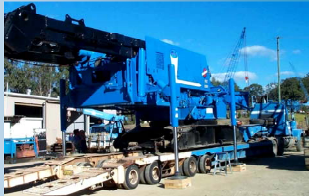
Above: M2250 being assembled by self erecting process.
