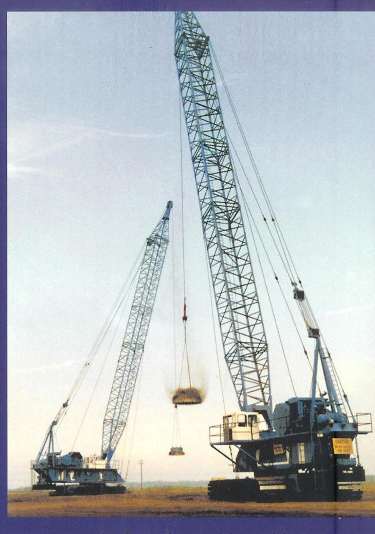
The Lampson LDC-350 Dynamic Compactor is a purpose-designed machine able to withstand the rigors of dynamic compaction work. Specifically engineered for vigorous duty cycle work it offers innovative features that reduce equipment wear and increase safety and ease of operation.
