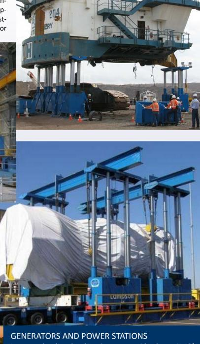
Lampson developed Jacking Systems provide alternative lifting solutions for lifting equipment from transport, for installation or for maintenance.
