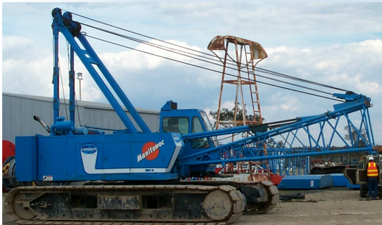
Above: The M50 with “X-Spander” attachment during pre-shipment tests at Lampson’s Toronto facility, NSW.
